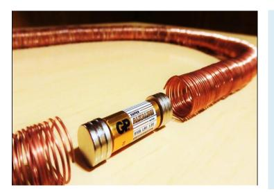
Magnets can also be use to create an electric train, on the left you can see a battery that has magnets attached on either end. Placing this inside a copper wire coil creates a magnetic field that allows the battery to move through the wire. This hints at how electric trains work. What is important about this type of train is that is does not produce any pollution!
